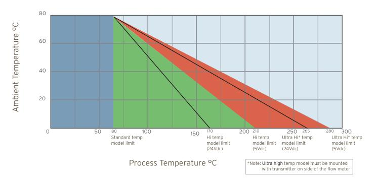
Temperature Limits Model 294 Transmitter Series
